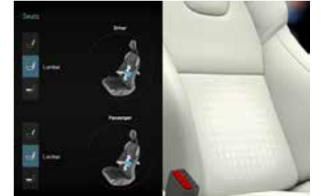
Power-operated multi-directional lumbar support
